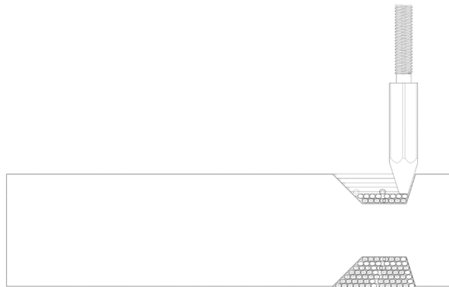
Figure 5 A detailed drawing of the nozzle, showing the wall taper
